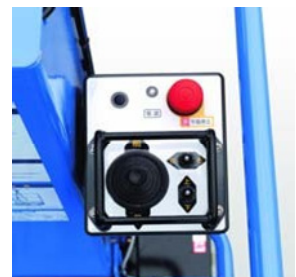
Photo: Upper control box
